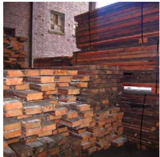
Floor planks salvaged from Harbor Island deconstruction site.
